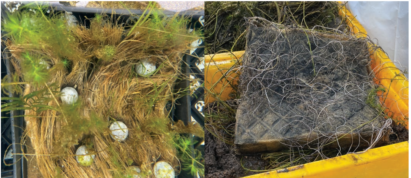
Native plants of milfoil and pondweed on a muka mat after approximately 6 weeks. Lead weights were used to hold the mat in place on plastic trays (that were buoyant) during this small-scale tank trial.
