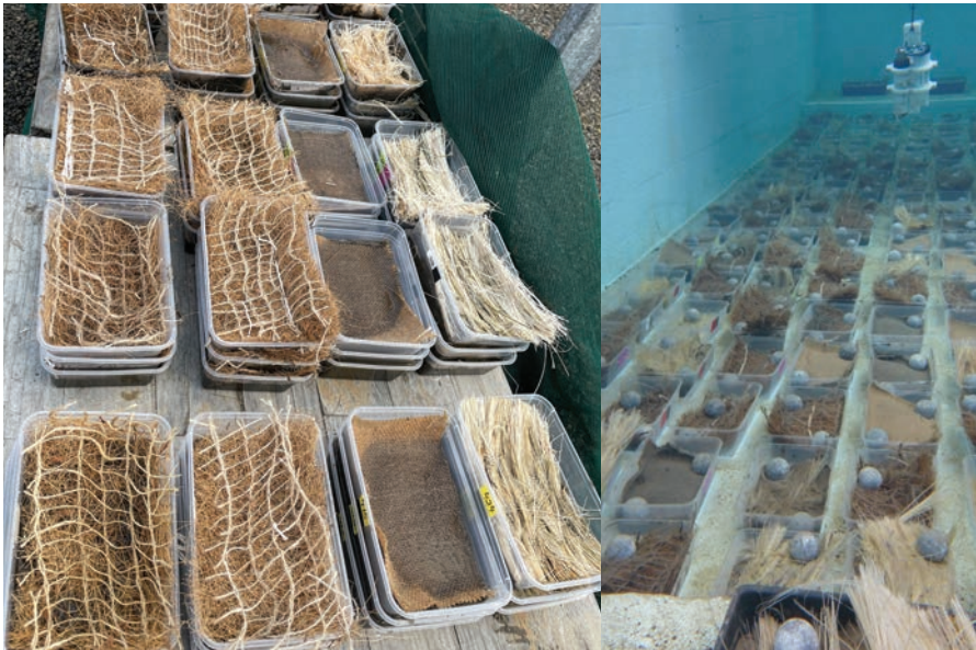
Photos: Before (left) and during (right) a mat degradation study where mat products were laid in trays with different substrates and placed in a tank to age. Every month for over a year the mats were assessed and tested to determine which products broke down the fastest.
