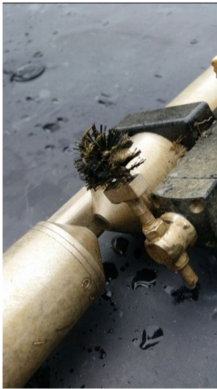
Traditional wire loop wiper brush from ZebraTech (photo: Evan Baddock, NIWA) versus a custom design (right, photo: Hamish Carrad, ECan).
